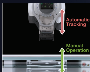
Motorized Vertical Synchronization with table, maintains constant SID
