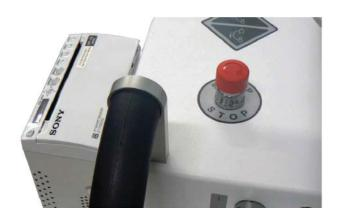
Optional, onboard thermal printer for output of procedure records.\*
