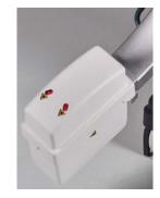
Zero dose centering with laser localizers on X-ray tube and flat panel detector.
